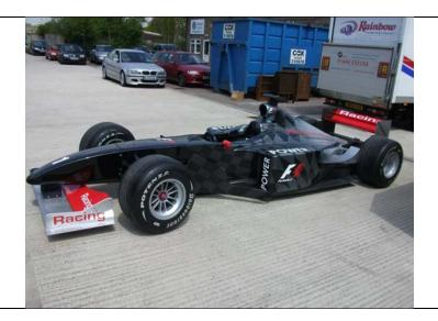
BAR F1 show car built with glass fibre chassis and many real parts ie rear wing bodywork some suspension parts
