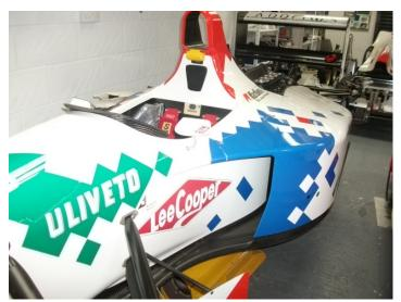
Footwork Arrows A14 this car raced in the 1993 F1 World Championship with Mugen V10 engines but they are not available and this example has been fitted with Hart DFR 3.5 litre engine.
